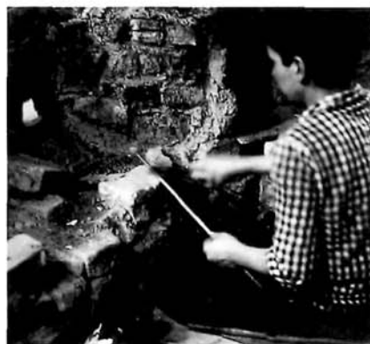
Plate 4. Winding a glass bead by inserting an iron mandrel into the hot glass in the furnace (furnace-winding). A few twists of the rod allow the glass to form into a bead shape which can be changed further by manipulation. This small glassworks is in Cairo, Egypt.
