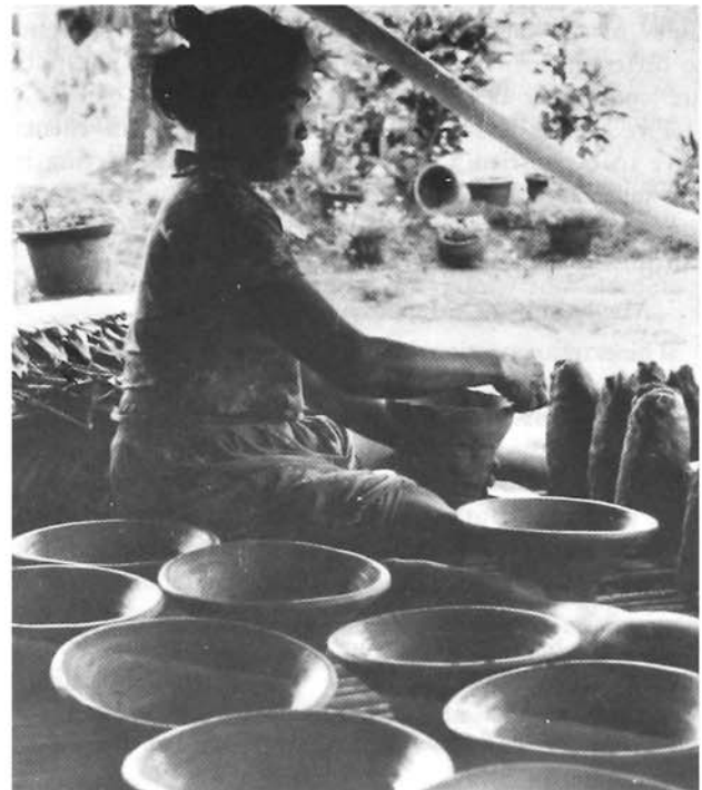
A potter at work. On the Foreground are partially worked vessels intended for flower pots. Techniques involve are hand-molding and paddle and anvil technique.
