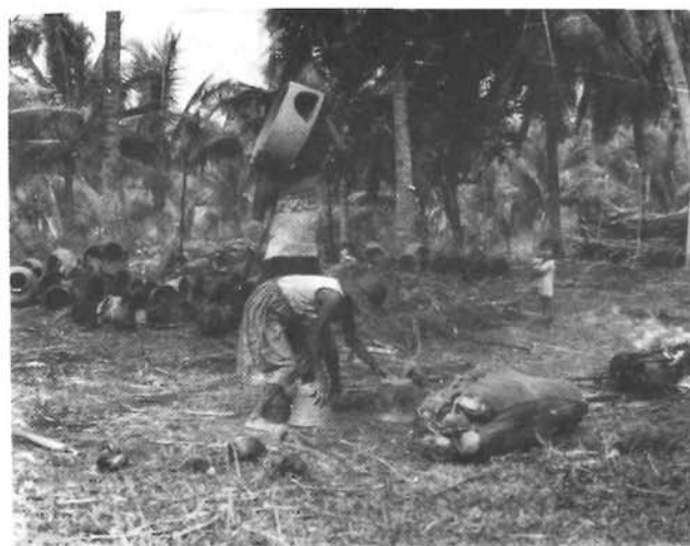
Open firing is a common sight in Bagacay especially on Saturdays. Every member of the family shares in this activity - gathering of firewood, pots' arrangement in the firing area, actual firing and packaging of pots.
