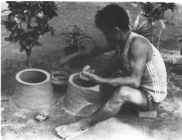
A male potter making a stove by hand-molding
