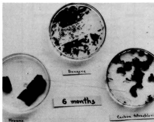
FIGURE 3. CURED LACQUER FILMS WERE SOAKED INTO NON-POLAR SOLVENTS FOR 6 MONTHS.
