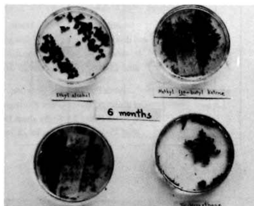
FIGURE 4. CURED LACQUER FILMS WERE SOAKED INTO POLAR SOLVENTS FOR 6 MONTHS.
