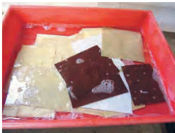
Figure 11: Soaked papers in sizing solution
