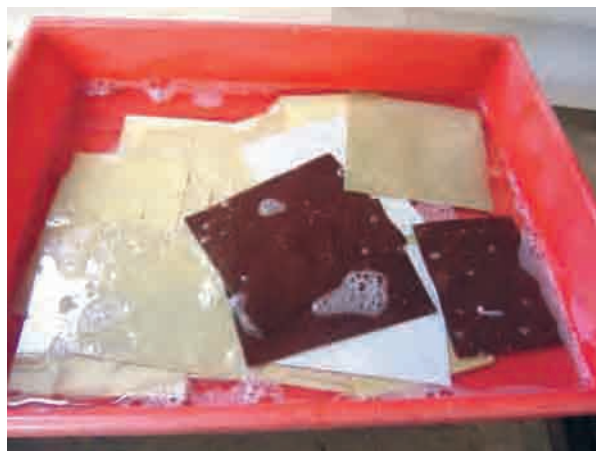
Figure 11: Soaked papers in sizing solution
