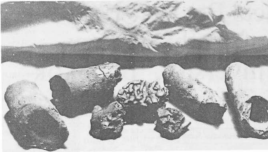
Remains of tuyere fragments showing slag wetted ends, vitrified and reduced areas along the sample; also shown are slag samples from the excavation at Ban Di Lung, Lopburi province (scale = 30 cm).
