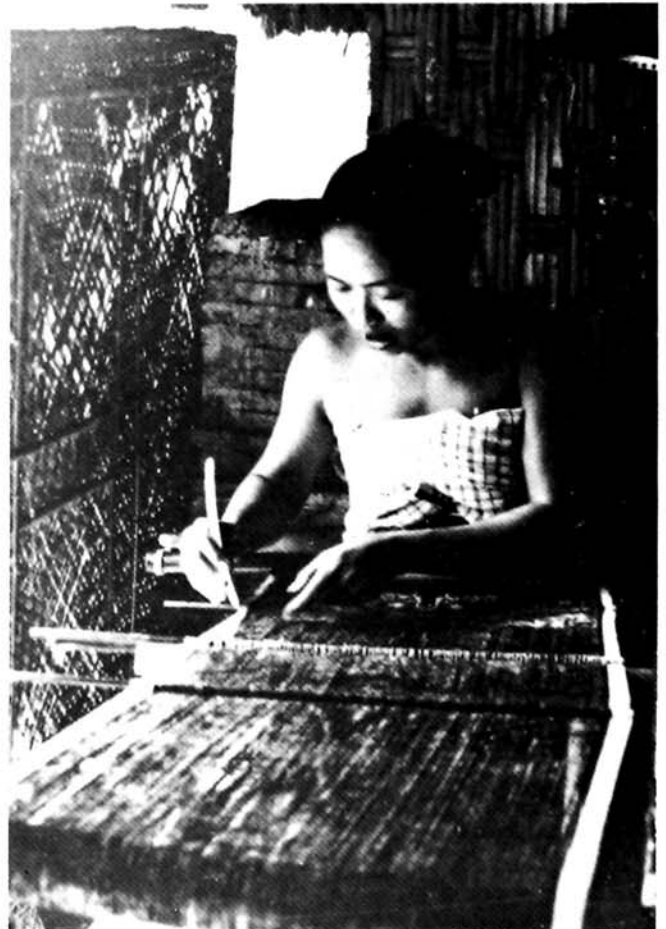
An Indonesian folk weaver working on a double weft ikat weave, with the traditional backstrap loom. Traditional weaving in the various countries of Southeast Asia, is performed as a ceremonial activity, before any weaving start.
