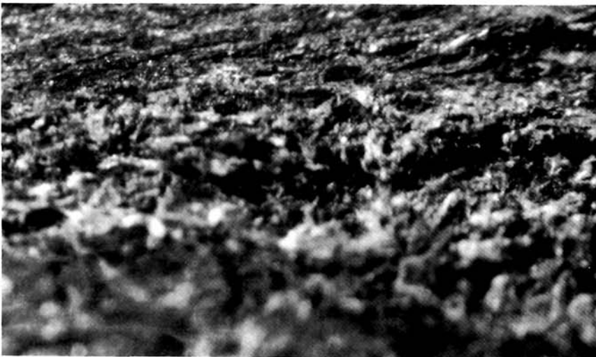
A cross-section of leather: On top is the grain side, showing dense fibre. At the bottom is the flesh, showing loose fibre.
