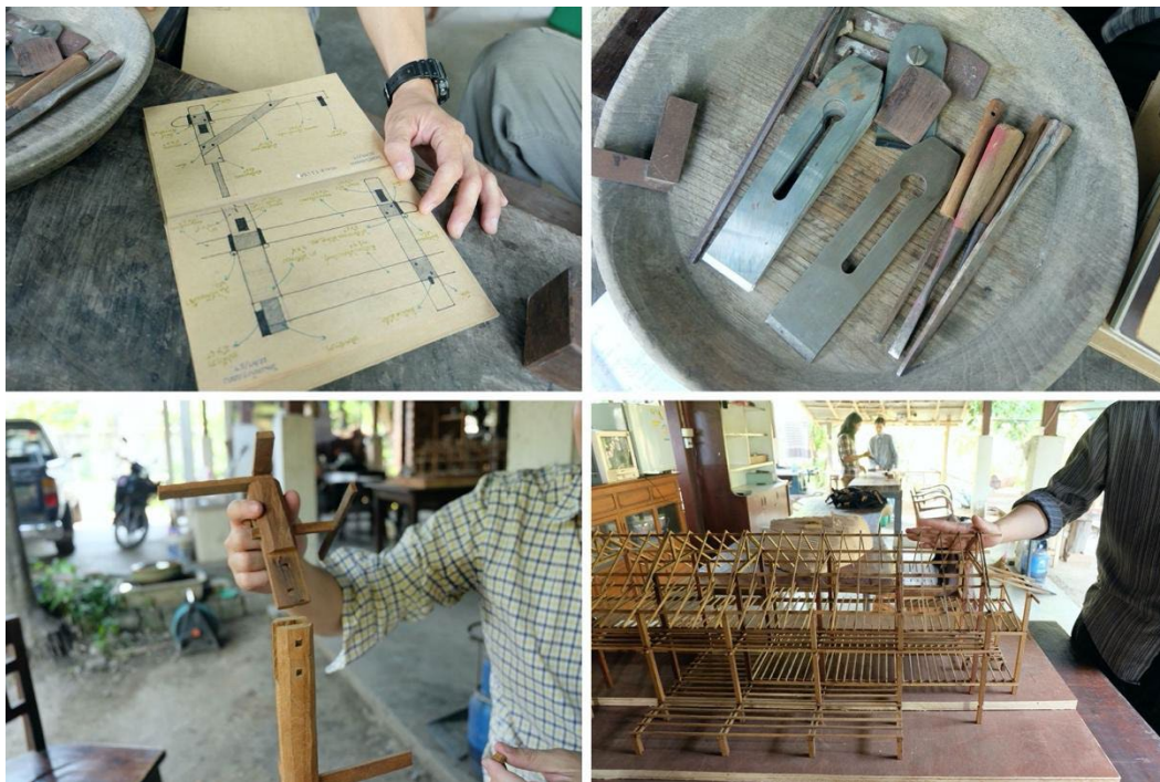
Fig. 11 (Upper left) The founders’ sketches of joinery, (Upper right) Hand tools they used in construction, (Bottom left) The joinery model they made after learning from a construction site, (Bottom right) One of the models of their projects. Source: Photo by Hiranpruek, 2016.
